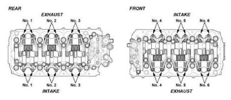
12. Insert the feeler gauge between the adjusting screw and the end of the valve stem on the No. 1 cylinder and slide it back and forth; you should feel a slight amount of drag.
