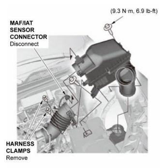
7. Disconnect the connector, then remove the harness holder.
